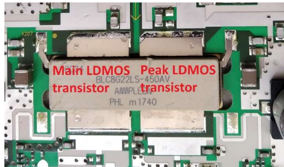
Figure 5. Double LDMOS used in final stage
